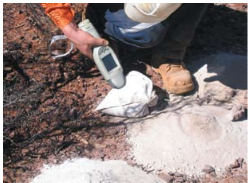
The NITON XLi 500 Series performing direct analysis on RC drill cuttings.
