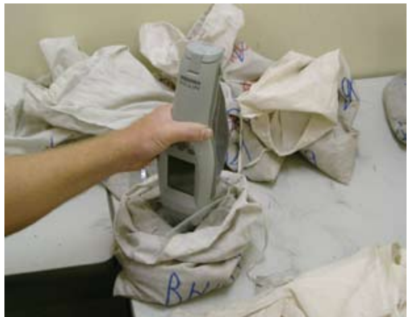
The NITON XLi 500 Series XRF analyzer testing unprepared blast hole cuttings.
